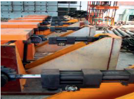
FIGURE 5: 1 m x 1 m 9-table seismic array of BJUT.
